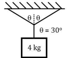
B. Use the diagram at right to determine the tension in Ropes I, II, and III.
