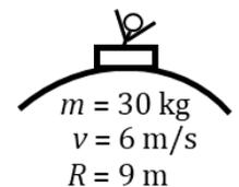
D. Now, the child is at the bottom of the next valley. Draw an FBD and determine the normal force of the hill on the sled.
