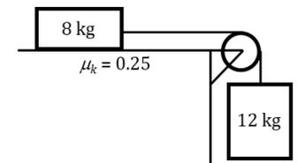
H. For the system shown, find the acceleration of the system and the string's tension.
