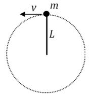
D. Suppose the stone in Part C is still moving at 8 m/s when it reaches the bottom of its path. Again, draw an FBD and determine the tension in the rope.
