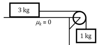
G. For the system shown, find the acceleration of the system and the string's tension.
