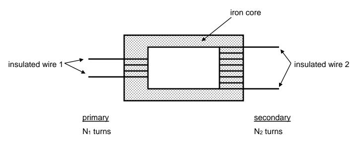
A <u>step-down transformer</u> the voltage;
