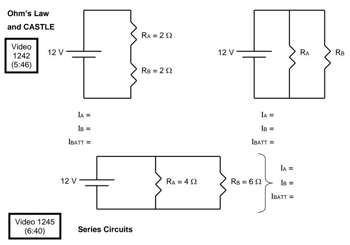
equivalent resistance: the resistance of several resistors taken together; it depends on the value of each resistor and on the configuration of resistors
