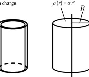
C. To analyze this charge distribution, we visualize the cylinder as a very large number of extremely thin coaxial cylindrical shells. The figure above represents one of these extremely thin shells. Into that figure, draw it having radius *r*, thickness *dr*, height *L*, and volume charge density *ρ*.
