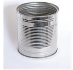
Many “tin” cans are actually Sn-coated steel.
